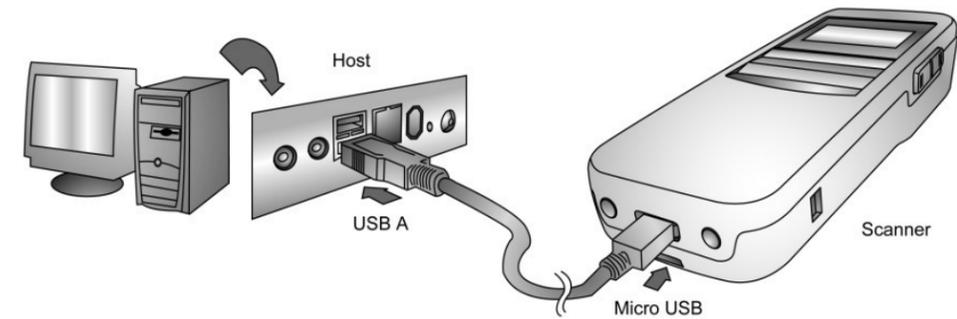
Insert the Micro USB cord into the scanner and into a USB port on the host PC. Charge for 4 hours.
